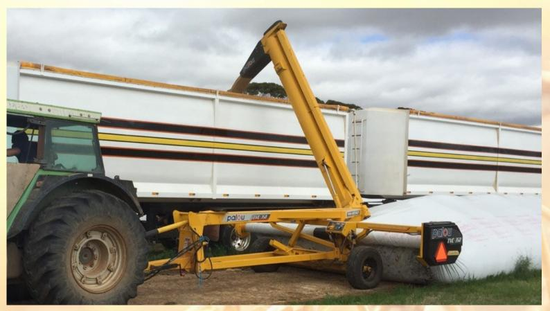
1. DISHARGE AUGER: Built in one piece, folds low and forward for transport. Being one piece means less grain damage, and significantly reduced auger wear and reduced power consumption overall.
