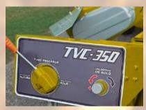
5. HYDRAULLIC CONTROLS: Requires only a single hydraulic circuit that is controlled by a by-pass valve for each control; volume regulating valve modifies bag rolling speed. Both controls are on a dashboard easily accessed by the operator without needing to get off the tractor to make changes.
